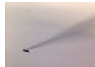
Adhesive forces hold the lamella to the glass needle
