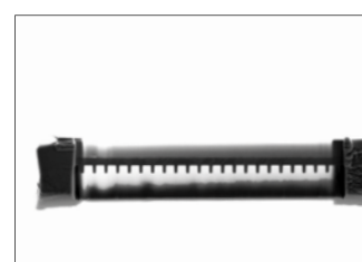
STEM detector image of the lamella
